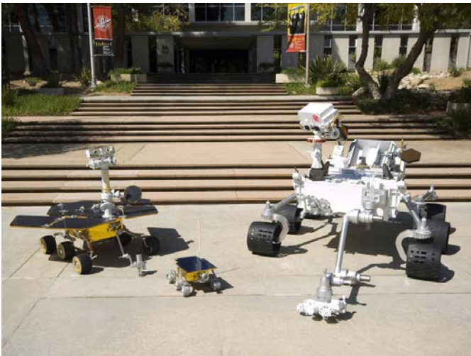
Figure 1. Mars rover family – Sojourner (1996) in the foreground, MER rover (2003) on the left, and MSL rover (2011) on the right
