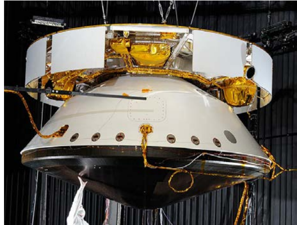
Figure 11. MSL Spacecraft in JPL 25-foot thermal Vac chamber
