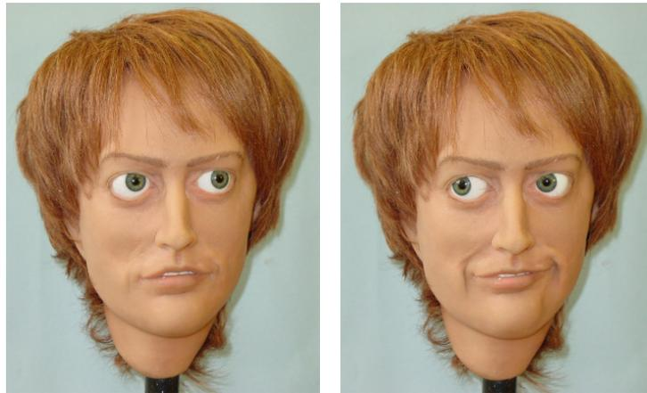
**Figure 1:** Using artificial skin provides an identity to a humanlike head and allows it to make facial expressions (made by David Hanson, Hanson Robotics, and photographed at JPL by the author).
