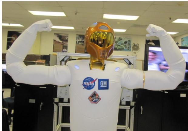
**Figure 2:** The Robonaut originally was developed as a tele-operated robot and it is currently being developed as an autonomous robot.
