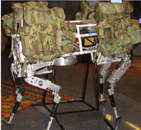
Figure 5: The Big-Dog (made by Boston Dynamics), which is a mull-like legged robot that was developed for military application. Photographed by the author.
