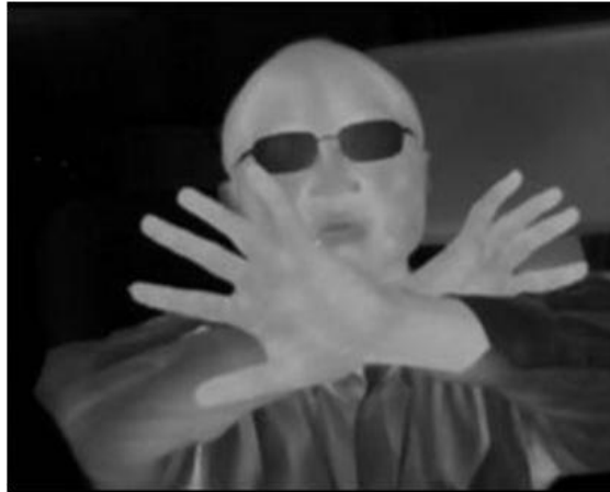
Figure 4. Image taken from a 320 x 256 CBIRD LWIR FPA at T = 80K. The FPA pixels were fully reticulated using the dry etch process described in this work.
