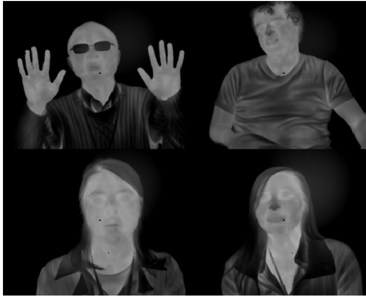
Figure 6. Images taken with a 320×256 format LWIR n-CBIRD focal plane array at an operating temperature of 78K. The detector cutoff wavelength is 10 \mu\text{m} .
