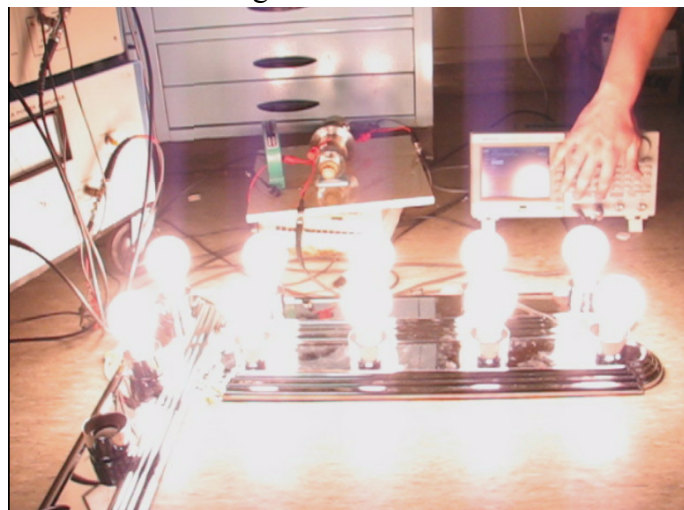
Figure 7. Ten 100W light bulbs powered by the wireless transmission device for ~5 seconds.
