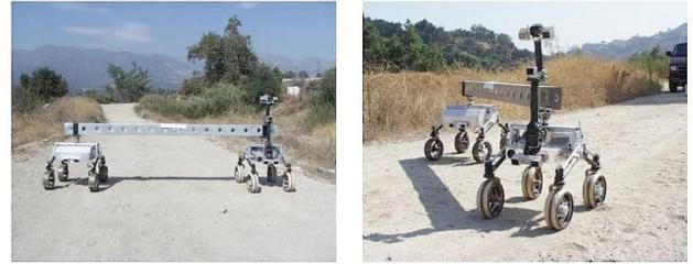
Figure 3. Coordinated transport of extended container (2.5 meters) by SRR and SRR2K, as performed in Arroyo Seco near JPL. (Left) row transport formation; (Right): column (leader-follower) transport formation
