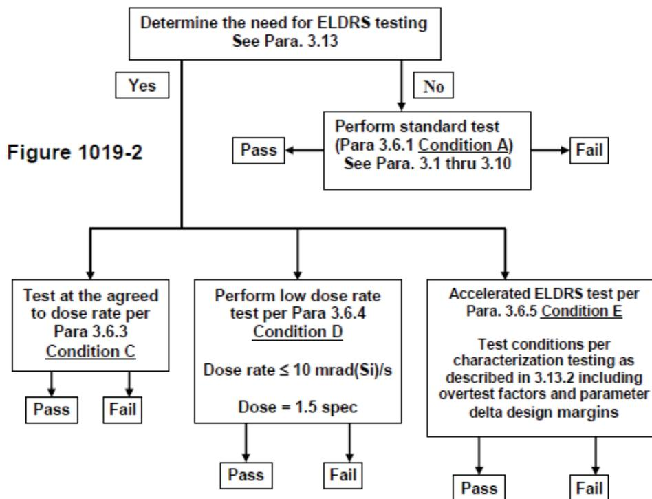
Fig. 10. Flow diagram for ELDRS testing from Test Method 1019.7
