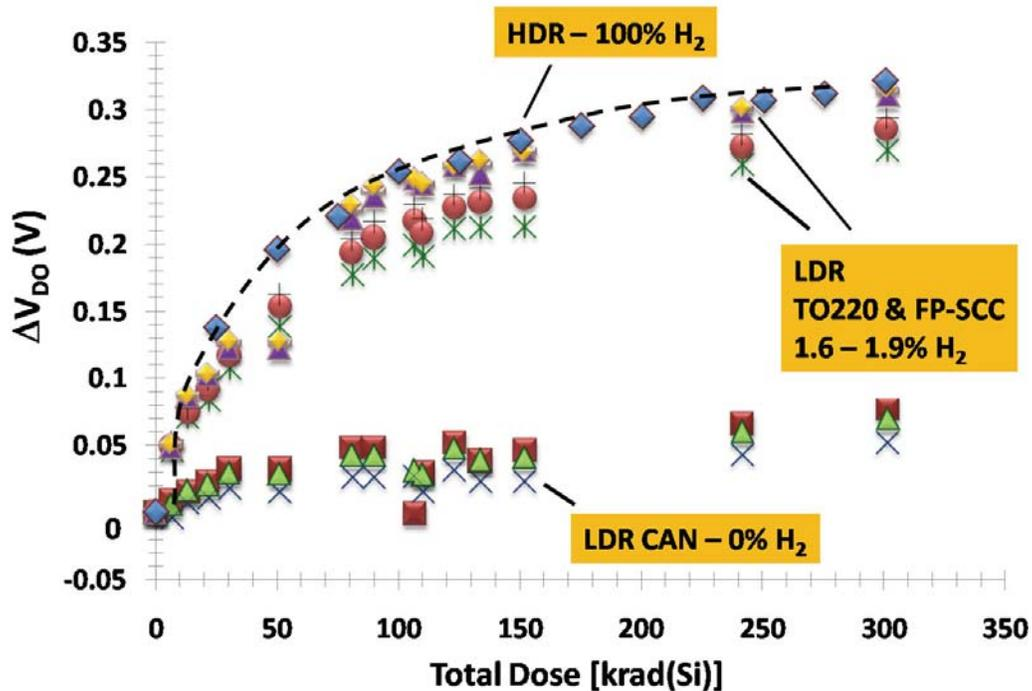
Fig. 5. Change in dropout voltage versus total dose for the HSYE-117 linear voltage regulator in three different packages (TO39, TO-220 and FP-SCC). Twelve parts were irradiated at LDR (0.05 rad/s). Two additional parts (TO-220) with the lid off were irradiated at HDR (50 rad/s) with 100% H<sub>2</sub>.
