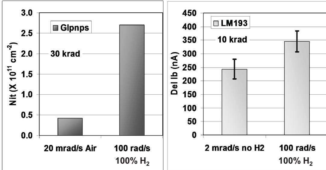
**Fig. 1.** Comparison of post irradiation interface traps ( $N_{it}$ ) for a GLPNP transistor irradiated to 30 krad(Si) at 20 mrad(Si)/s in air to irradiation at 100 rad(Si)/s in 100% H<sub>2</sub> (left) and delta Ib of an LM193 from National Semiconductor to 10 krad(Si) at 2 mrad(Si)/s in air to irradiation at 100 rad(Si)/s in 100% H<sub>2</sub> (right).
