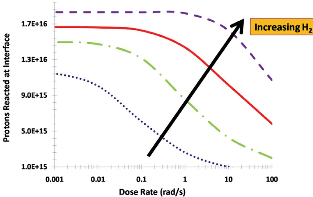
Fig. 2. Protons reacted at interface at 30 krad as a function of dose rate for different hydrogen levels based on the model defined by equation 3.
