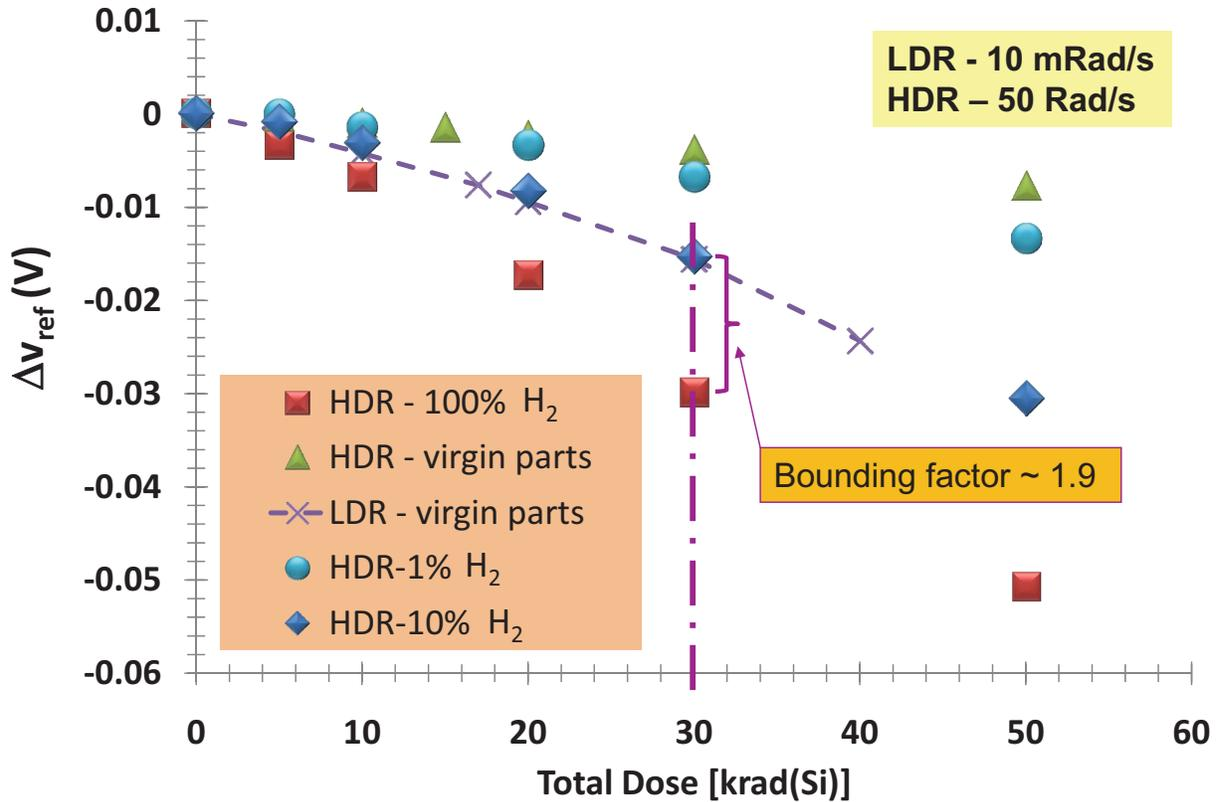
Fig. 4. Change in reference voltage for the LT1019 as a function of total dose for four irradiation conditions: HDR (50 rad/s), LDR (10 mrad/s) and (50 rad/s with 1, 10 and 100 % H<sub>2</sub>).
