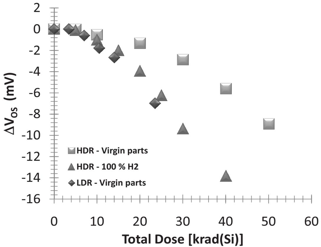
Fig. 7. Change in offset voltage versus total dose for the Analog Devices OP42. The HDR results are shown for irradiation at 50 rad/s (HDR – virgin parts) and 1 rad/s in 100% H<sub>2</sub> (HDR – 100% H<sub>2</sub>), as well as a LDR result at 0.04 rad/s (LDR- virgin parts).
