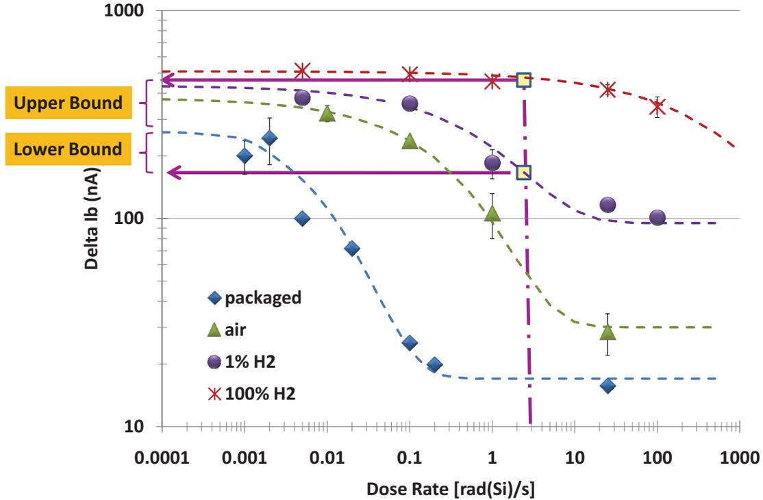
Fig. 3. Increase in input bias current vs dose rate for irradiation to 10 krad for the LM193s, with p-glass and different % H<sub>2</sub> and for nitride with no H<sub>2</sub>. At 1 rad/s the 1% H<sub>2</sub> underestimates the low dose rate response whereas the 100% H<sub>2</sub> bounds it.
