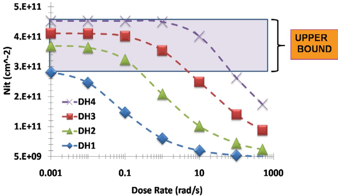
Fig. 8. Simulation of  $N_i$  formation as a function of dose rate for different hydrogen concentrations. Simulations capture the right shift of transition dose rates and the increase of low dose rate saturation limit. In these simulations,  $DH4 > DH3 > DH2 > DH1$  and  $\sigma4 < \sigma3 < \sigma2 < \sigma1$ .
