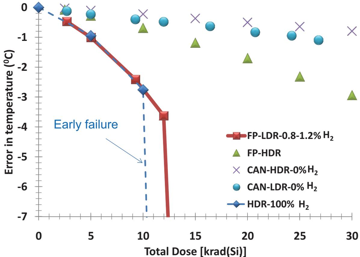
Fig. 6. Degradation of the AD590 temperature error as a function of total dose. Two groups of three flatpacks and three cans were irradiated unbiased at both high and low dose rate (respectively 25 rad/s and 0.01 rad/s). RGA was performed after irradiation on the flatpack devices to evaluate the amount of hydrogen. Three additional parts (cans) with the lid off were irradiated at HDR (1 rad/s) with 100% H<sub>2</sub>.
