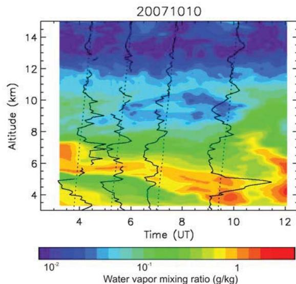
**Figure 4:** Time-altitude 2D color contour plot of water vapor mixing ratio measured by the JPL lidar on the night of October 10, 2007. The superimposed black solid curves represent the departure from nightly mean as measured by the four radiosondes launched on that night. The black dotted lines show the time-altitude position of the balloon, and the zero-departure in water vapor.
