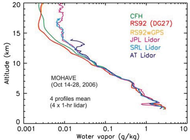
**Figure 1:** Mean of four water vapor profiles simultaneously measured by CFH, three lidars, and two RS92 radiosonde systems during MOHAVE.
