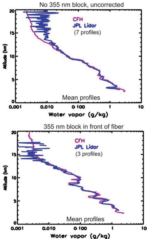
**Figure 2:** Mean water vapor profile measured simultaneously by CFH and by the JPL lidar. a) measured with the lidar original configuration. b) measured with a 355-nm blocking filter in front of receiver
