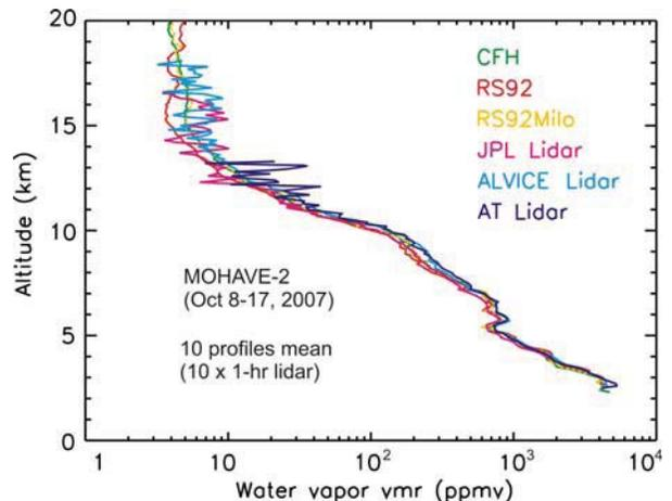
**Figure 3:** Mean water vapor profile simultaneously measured by CFH, three lidars, and RS92 radiosonde during MOHAVE-II.
