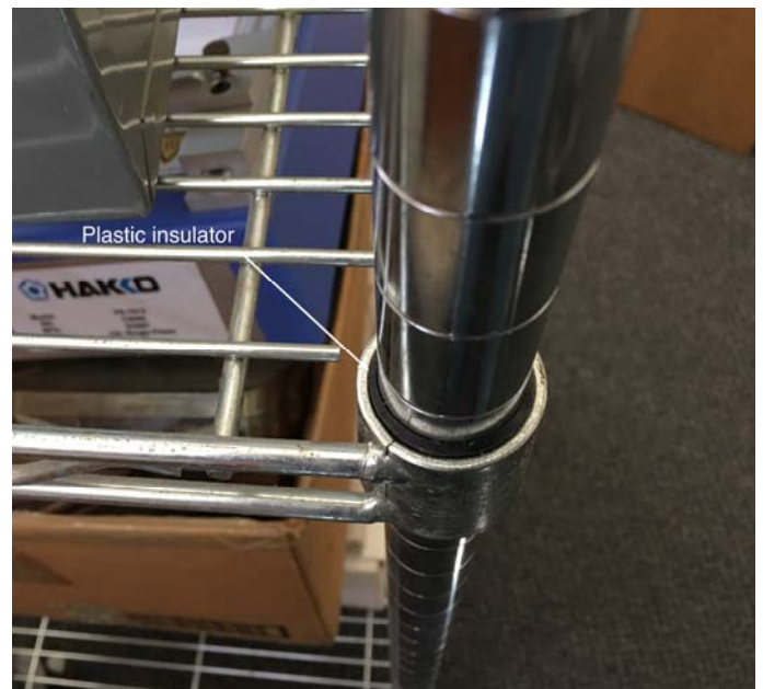
Figure 2. Photograph showing a plastic insulator inserted at each connector junction in a storage rack. Such rings prevent grounding of items stored on the rack. Lack of grounding could lead to build-up of a damaging electrostatic charge. (Figure courtesy of Steve Bolin.)
