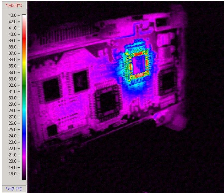
Short-wave infrared image showing an application-specific integrated circuit (ASIC) that had a bus contention problem at a low temperature causing it to malfunction. An infrared camera placed inside the oven precisely located the device failure point when the downward-cycling oven reached 16°C. The device was later replaced, and the spacecraft hardware worked throughout the mission.
