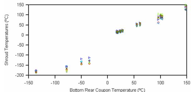
**Figure 11. Shroud Temperatures vs Bottom Rear Heat Flux Sensor Temperature at Steady-State.**
