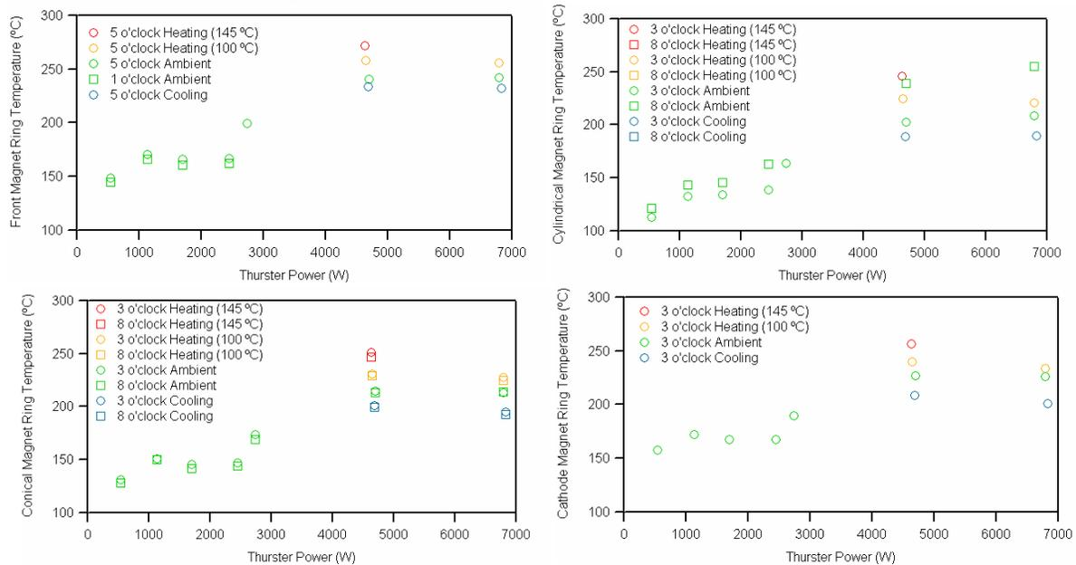
**Figure 12. Steady-State Magnet Temperatures During Thermal Development Testing**
