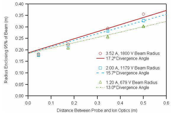
**Figure 10. Beam Divergence During Post-TDT Functional Testing**
