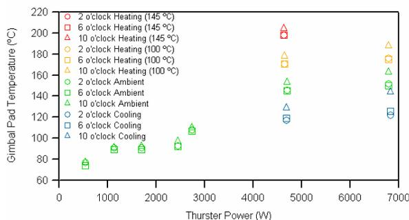
**Figure 17. Steady-State Gimbal Pad Temperatures During Thermal Development Testing**
