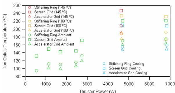
**Figure 16. Steady-State Ion Optics Temperatures During Thermal Development Testing**
