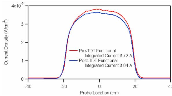
**Figure 9. Comparison of Pre- and Post-TDT Functional Faraday Probe Data at 1800 V, 3.52 A**
