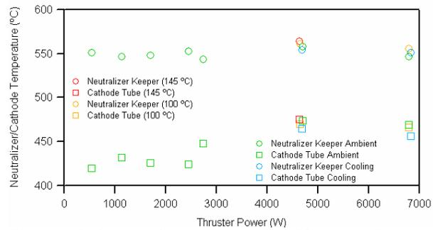
**Figure 19. Steady-State Neutralizer/Cathode Temperatures During Thermal Development Testing**
