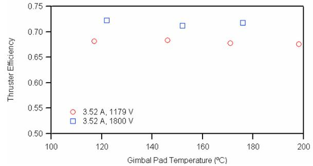
Figure 22. NEXT PM1 Efficiency Over the Thermal Range
