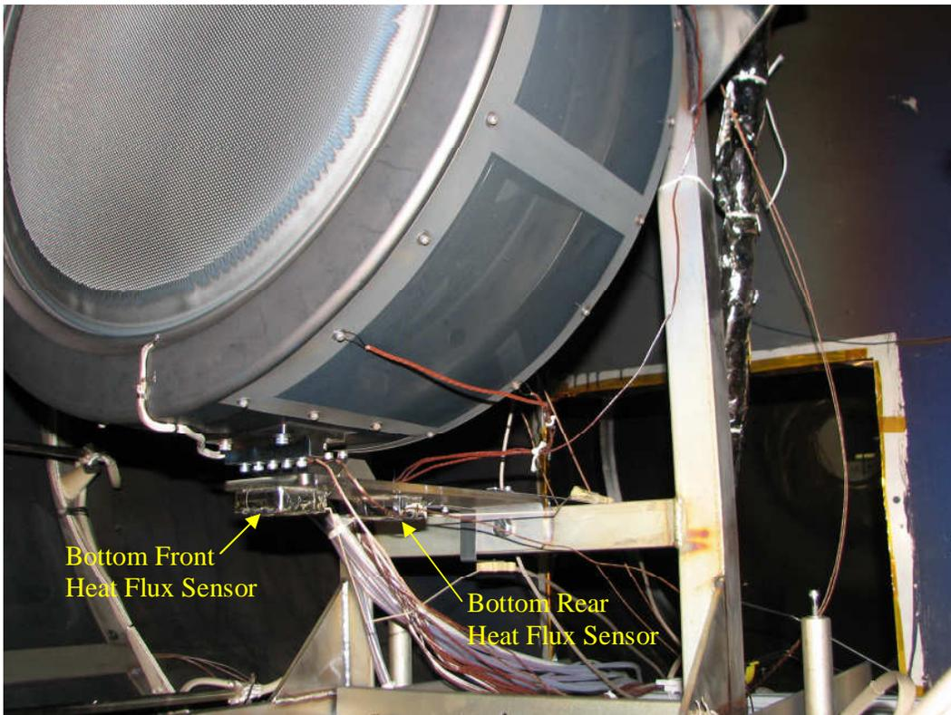
**Figure 4. NEXT PM1 and Bottom Heat Flux Sensors.**
