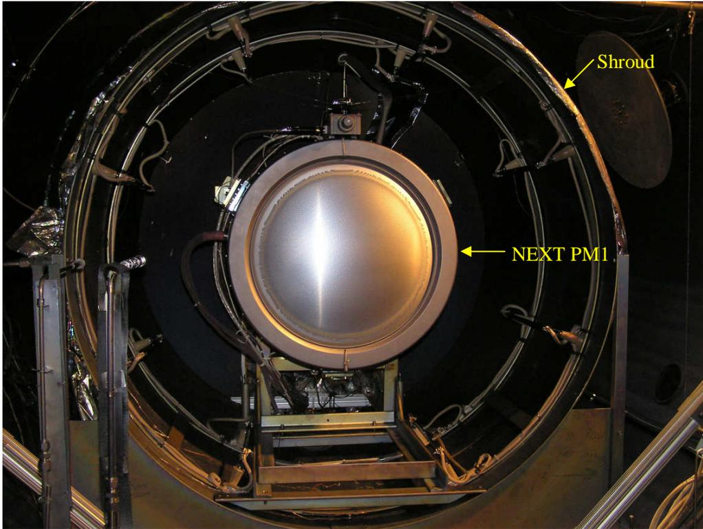
**Figure 2. NEX T PM1 Installed Inside Thermal Shroud.**
