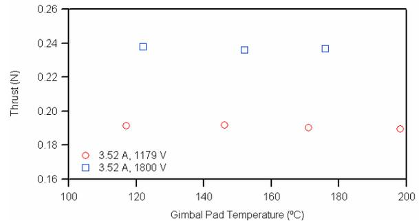
**Figure 20. NEXT PM1 Thrust Over the Thermal Range**
