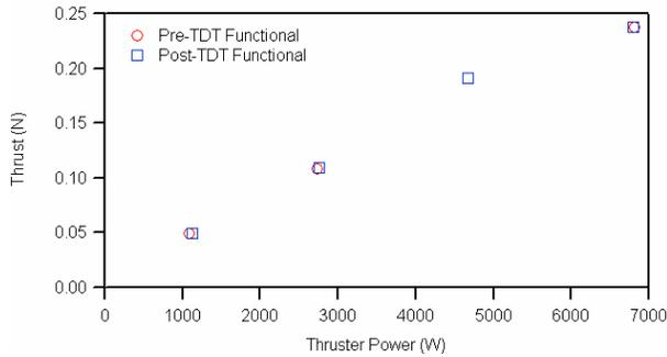
**Figure 6. NEXTPM1 Thrust vs Power During Functional Testing**
