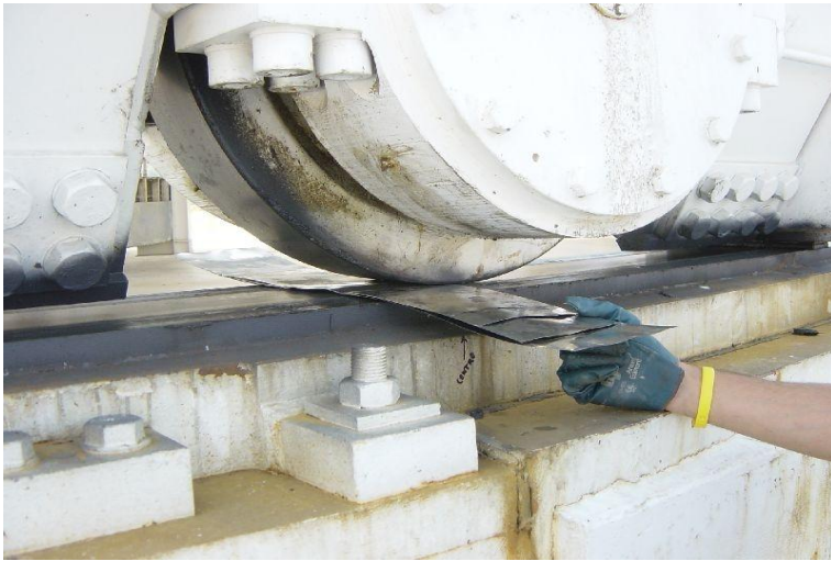
Figure 10. Azimuth wheel crosses 1mm shim
