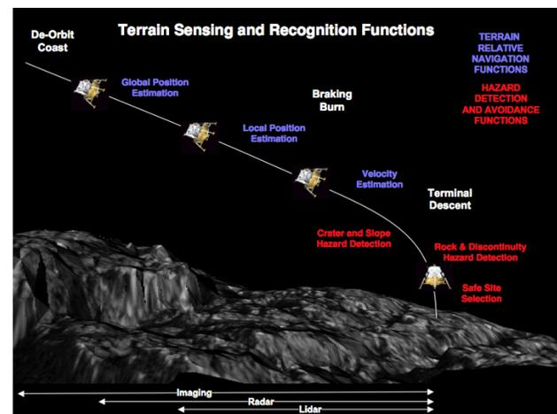
**Figure 1: Terrain sensing and recognition functions for safe and precise lunar landing.**
