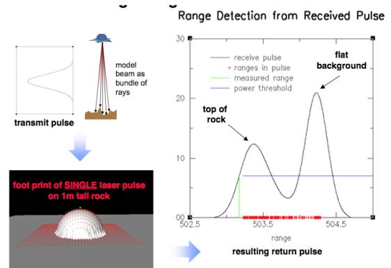
Figure 3: Ranging model used in LIDAR simulator.
