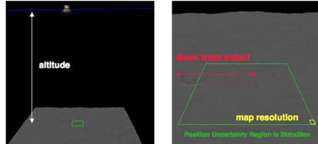
**Figure 5: Parameters investigated in Altimeter to DEM Correlation simulation.**
