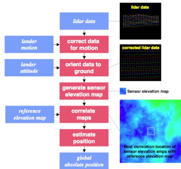
Figure 4: Active ranging TRN algorithm block diagram.
