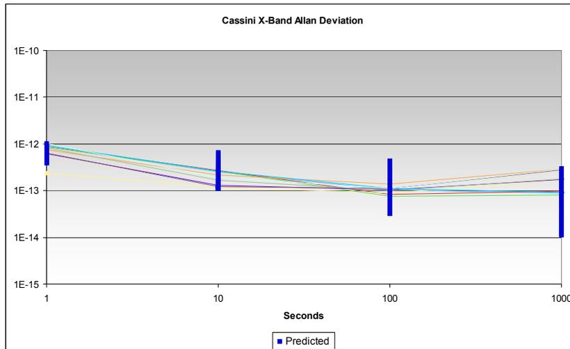
**Figure 13. Frequency stability between observed and model**
