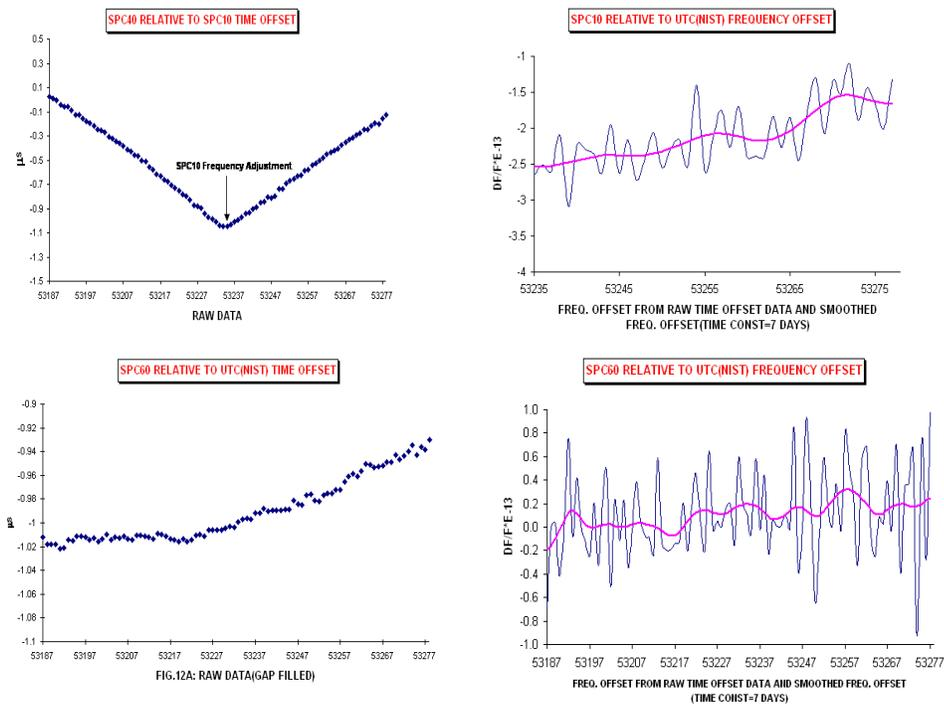
Figure 16. Frequency and timing synchronization offset
