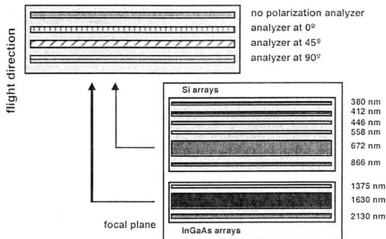
Figure 2. Conceptual focal plane layout for the integrated sensor. Like MISR, each camera would contain a focal plane containing linear arrays, so that imagery is acquired in pushbroom fashion. However, a greater number of spectral bands is envisioned, and in two bands (one visible and one shortwave infrared), polarization measurements would be acquired. The detector material is Si for the wavelengths shortward of 1  $\mu\text{m}$ , and InGaAs for the remainder.
