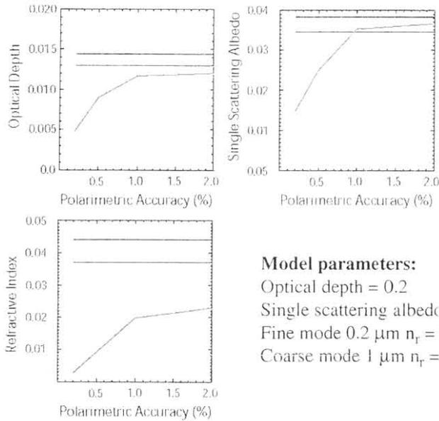
Figure 1. Sensitivity to optical depth, single scattering albedo, and real part of the refractive index as a function of accuracy in measurement of *DOLP*.
