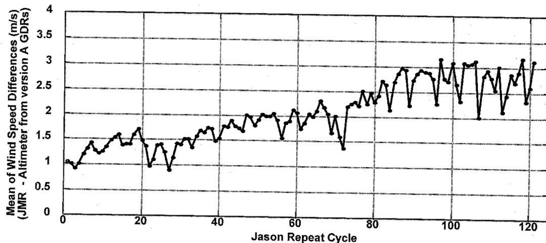
Figure 3. JMR – Altimeter wind speed retrievals for first three years of mission.
