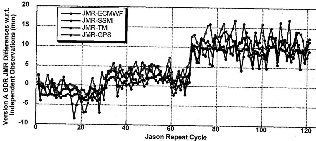
Figure 2. 10-day global averaged JMR path delay compared to various sources of ground truth.
