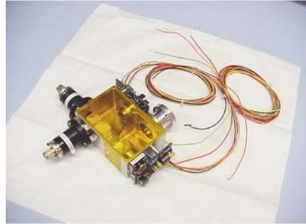
Fig 7. Vertex-to-vertex beam launcher
