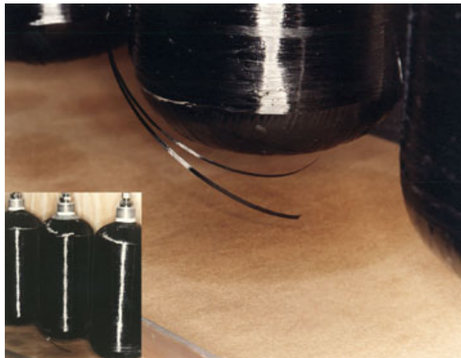
Figure 3. Fiber tow failure on test vessel.
