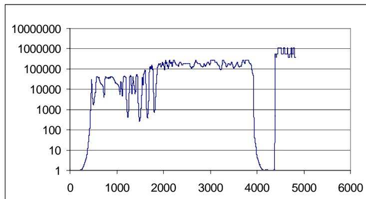
**Figure 4.** The Achromatic Nuller Testbed (ANT) has produced nulls with a 200,000:1 null achieved in 10  $\mu$ m laser light and a 15,000:1 null at 25% bandwidth.
