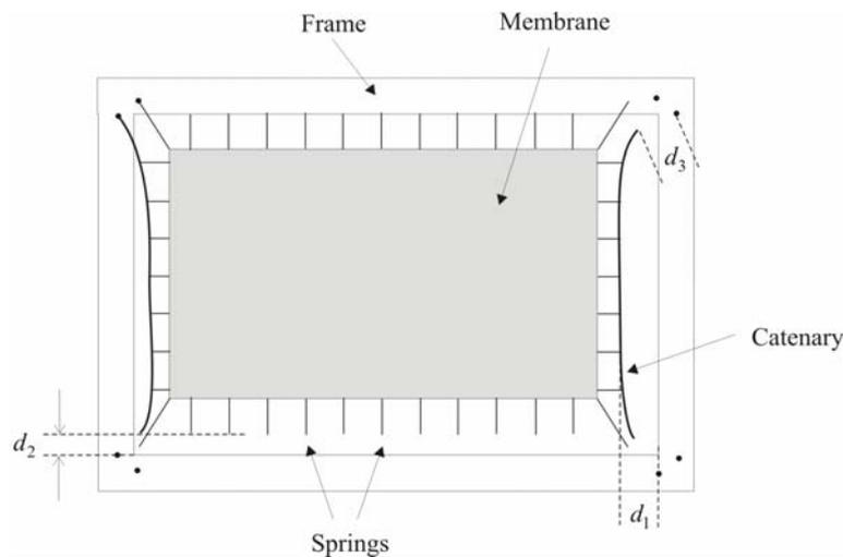
Figure 2 – Schematic of frame-membrane assembly
