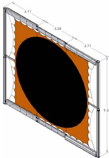
*Figure 1 – Design drawing of the eight-meter diameter membrane antenna*
