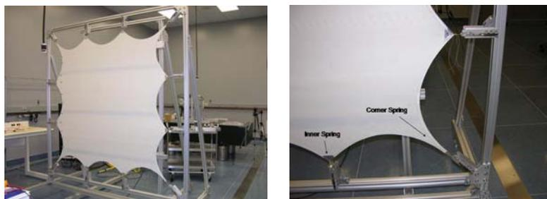
Figure 3 – Test setup(left),close up at tensioning springs (right)
