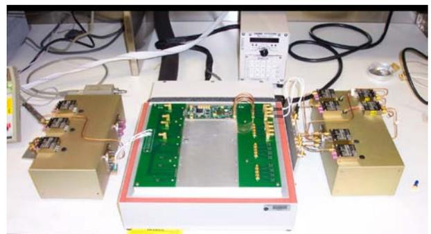
Fix xxx. Automated Test Station Hot-Cold Plate and RF Switching
