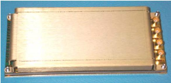
Fig xxx. T/R Module with Baseplate and Lid
