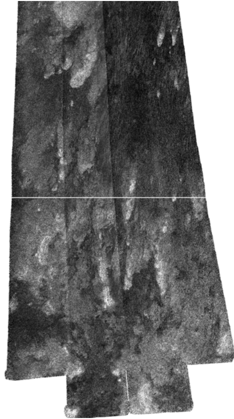
Figure 5. Latest acquired portion of T8 swath. (10-18 minutes after periapsis) White line indicates where the iso-doppler SAR swath would have ended.
