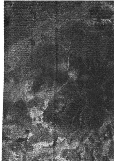
Figure 3. Portion of TA SAR swath near closest approach processed with the best available ephemeris and attitude data. No range and Doppler tracking applied.
