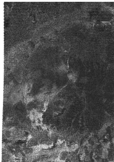
Figure 3. Portion of TA SAR swath near closest approach processed with the best available ephemeris and attitude data. No range and Doppler tracking applied.
