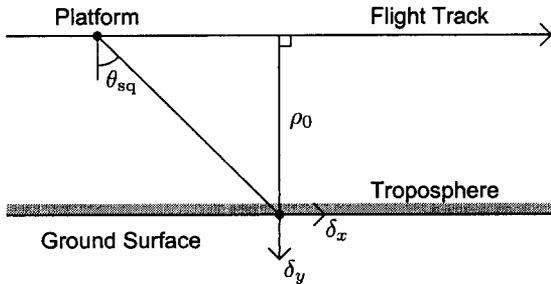
Figure 1: Geometry for the model used to describe the performance of the multisquint technique. The plane of the page corresponds to the slant plane.
