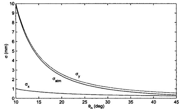
Figure 3: RMS displacement error and tropospheric path delay error for various values of  $\theta_0$  with the same system parameters assumed for Table 1. Note that  $\sigma_n$  has been kept fixed for all values of  $\theta_0$ .
