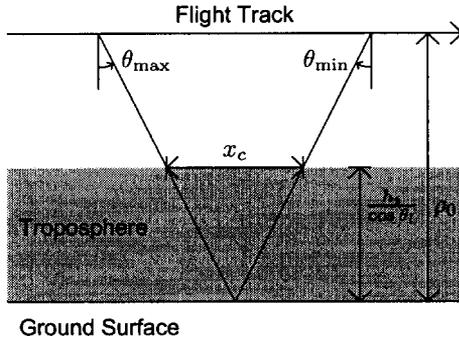
Figure 2: Geometry for computing the ray-path separation  $x_c$  at the effective top of the troposphere. The plane of the page represents the slant plane, oriented at an angle  $\theta_l$  from vertical.
