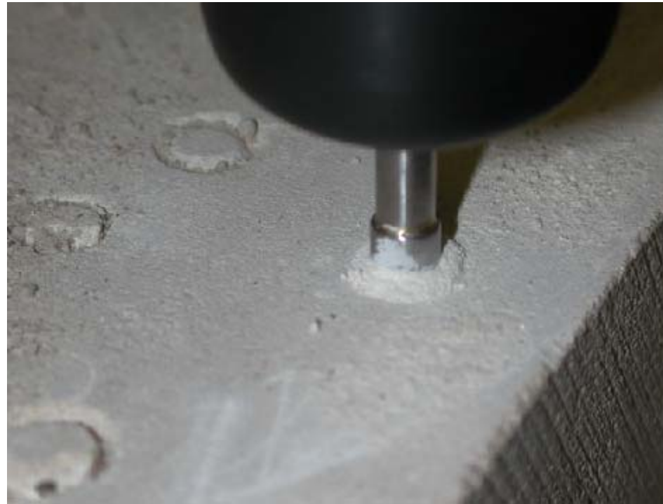
The sampler in action drilling limestone and accumulating powdered cuttings inside the bit
