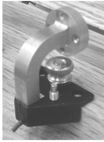
Fig. 2. Photograph of the GGB Industries WR3 Model 325 on-wafer probe with integrated bias tee.
