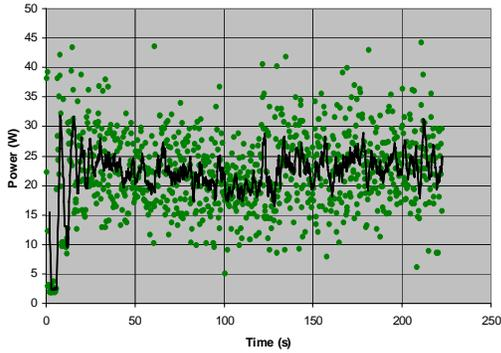
**Fig. 6:** Input power of the transducer, the dots are data points and line is the average.
