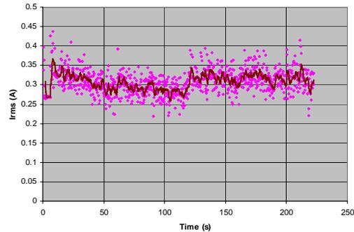
Fig. 5: Input current of the transducer, the dots are data points and line is the average.
