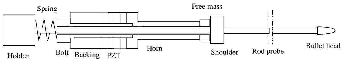
**Fig. 2:** Sketch of the structure of the prototype soil penetrator
