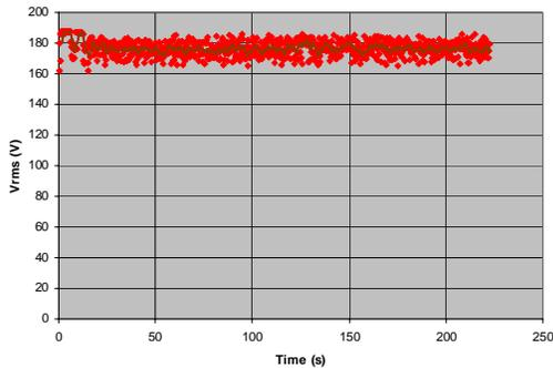
Fig. 4: Input voltage of the transducer, the dots represent data points and line is the average.
