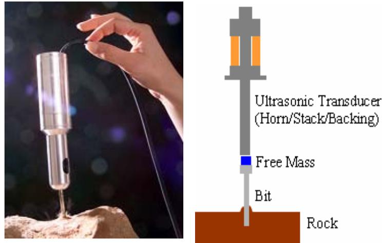
**Fig. 1:** A photographic view of the USDC showing its ability to core with minimum axial force (left), and a schematic diagram of its cross-section (right).
