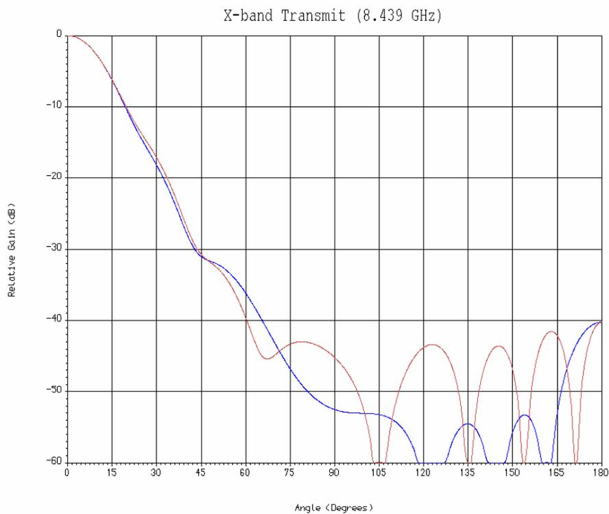
Figure 2. E- and H-plane Feed Patterns at 8.439 GHz
