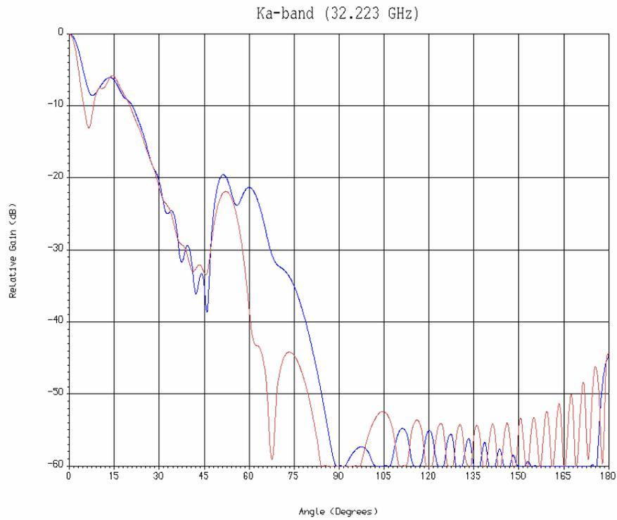
Figure 3. E- and H-plane Feed Patterns at 32.223 GHz
