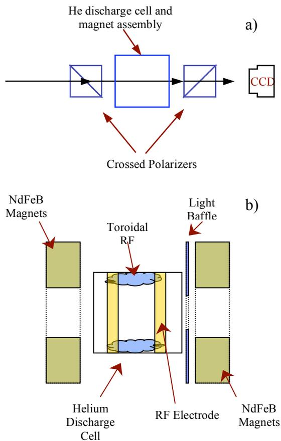
Figure 1 a) The overall layout of the test instrument showing the helium cell and magnet assembly placed between crossed polarizers. The arrows show the optical axis, which is parallel to the magnetic field. b) Details of the helium cell and magnet assembly, showing the placement of the magnets relative to the discharge cell.
