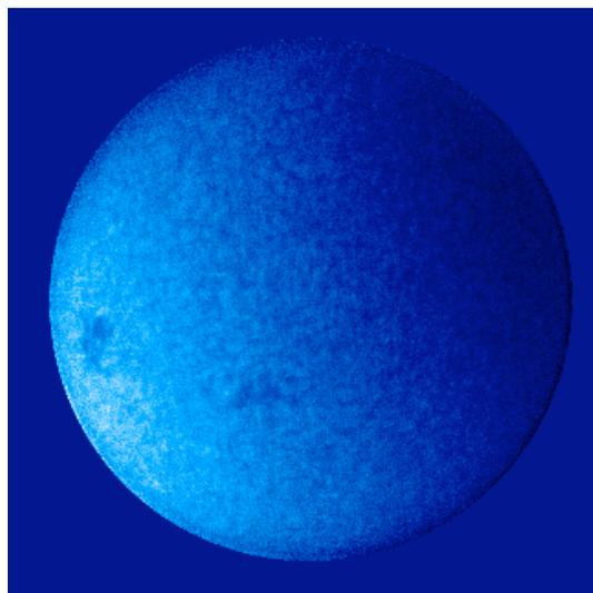
*Figure 3. A Doppler image produced by a Calcium 422.7nm magneto-optical filter. The Calcium 422.7 MOF, together with the He 1083nm MOF will form part of the MOTH II experiment.*
