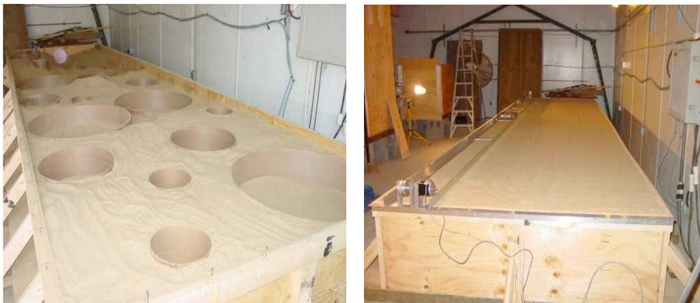
**Figure 3. HYDRA/SNeuP test setup at the Cold Regions Research Engineering Laboratory (CRREL). (Left) Construction of buried ice-bearing deposits in otherwise dry soil. (Right) Final configuration with motorized sled apparatus for performing traverses at -40° C.**
