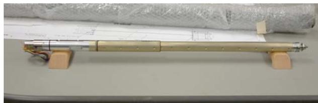
**Figure 2. D-HYDRA Drill-Integrated Neutron Spectrometer.**
