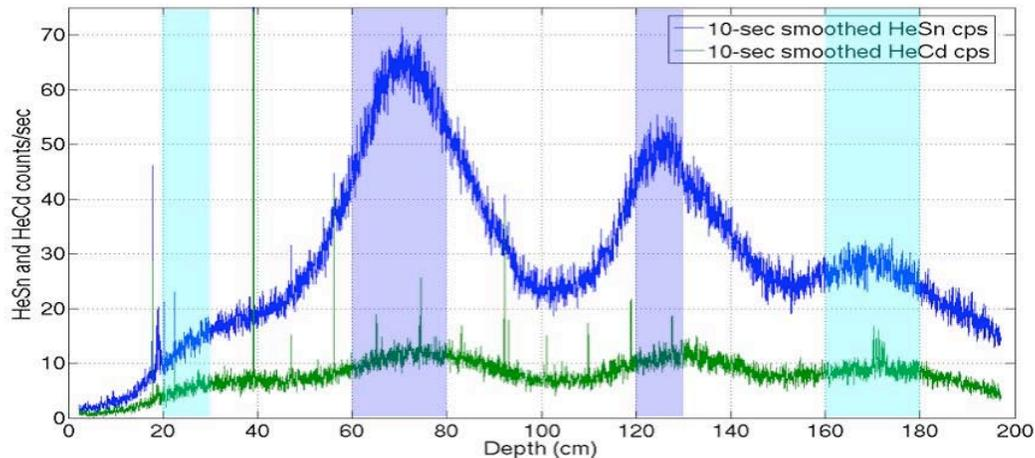
**Figure 6.** Running 10-sec averages of D-HYDRA count rates in the HeCd epithermal (green) and HeSn thermal+epithermal (blue) energy ranges versus depth for the test depicted in Figure 5. Data from CRREL on October 12, 2005.
