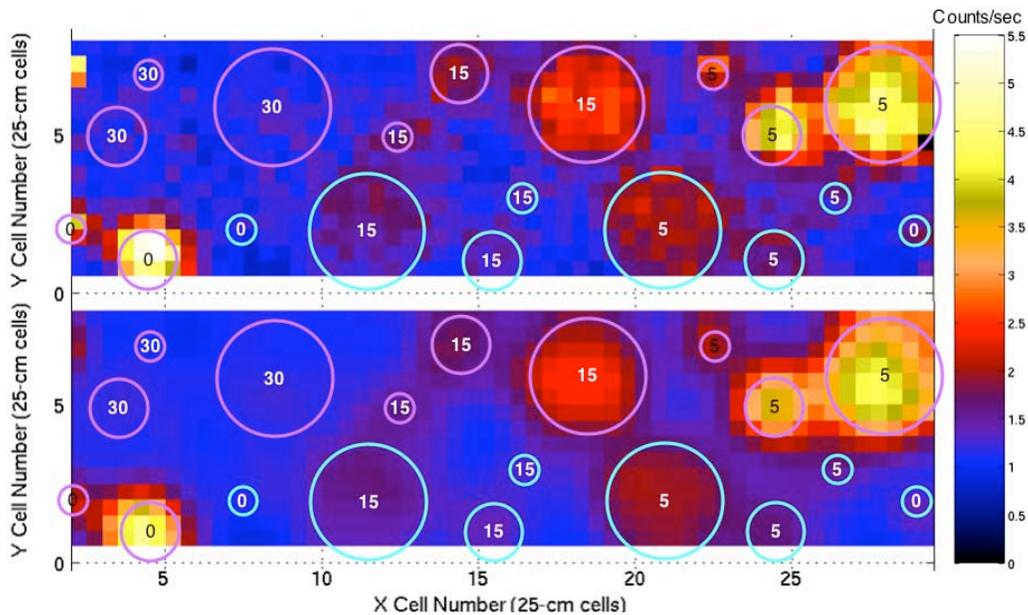
**Figure 4. (Top) HeSn (thermal+epithermal) count rates binned in 12.5 cm square bins. (Bottom) HeSn count rates binned and smoothed using a gaussian with a 26-cm full-width at half-maximum. Icy deposit outlines are superimposed; numbers indicate depth of burial. Data from CRREL testing, 3-7 October, 2005.**
