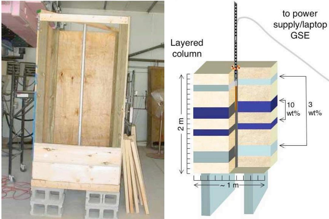
**Figure 5. (Left) The D-HYDRA/BNeuP borehole test setup during construction at CRREL. The borehole tube is at the center. (Right) Schematic showing borehole stratigraphy, comprised of alternating wet (3 and 10 wt% H<sub>2</sub>O) and dry (0.5 wt% H<sub>2</sub>O) layers.**
