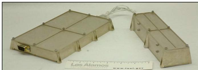
**Figure 1. HYDRA Neutron Spectrometer Version 2.0.**
