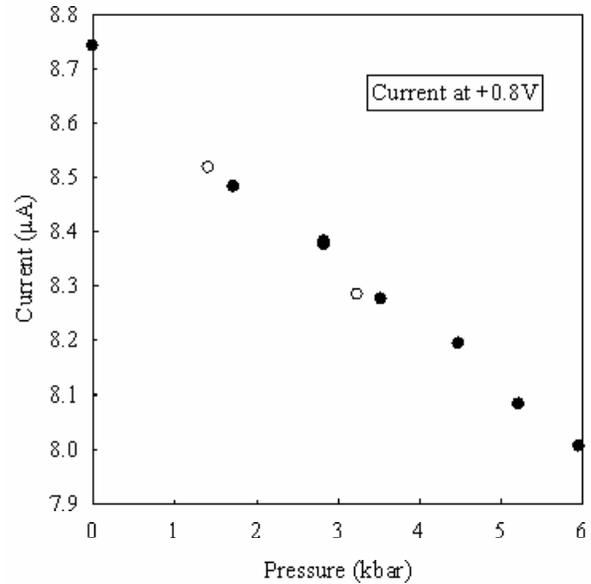
Figure 5. Pressure response measured for the n-GaN/ $\text{Al}_{0.15}\text{Ga}_{0.85}\text{N}$ /n-GaN single barrier vertical transport device. Current was measured under hydrostatic pressure at a fixed forward bias (+0.8 V) while the pressure was increased (solid dots) and decreased (open dots) as well. Linear decrease of the current with increasing pressure was observed and the response was reversible.
