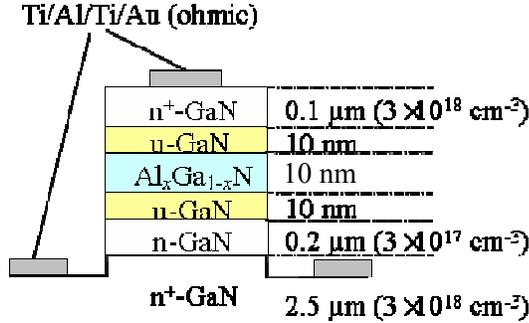
Figure 3. Schematic of the n-GaN/ $\text{Al}_x\text{Ga}_{1-x}\text{N}$ /n-GaN (nIn) devices investigated.
