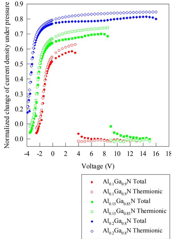
Figure 2. Modeling of normalized change of total and thermionic current densities,  $(J-J_0)/J_0$ , of n-GaN/ $\text{Al}_x\text{Ga}_{1-x}\text{N}$ /n-GaN heterojunction under 10 Kbar hydrostatic pressure. Both GaN layers are assumed to have a doping concentration of  $5 \times 10^{17}/\text{cm}^3$ , and 10 nm thick undoped  $\text{Al}_x\text{Ga}_{1-x}\text{N}$  is assumed. The bottom GaN surface is set as ground.
