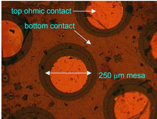
Figure 4. Optical image of n-GaN/ $\text{Al}_{0.15}\text{Ga}_{0.85}\text{N}$ /n-GaN heterojunction devices used for pressure measurements. The heterostructure was grown on a SiC surface using MOCVD. The  $\text{Al}_{0.15}\text{Ga}_{0.85}\text{N}$  layer was undoped and 10 nm thick. The diameter of the heterojunction mesa structure is 250
