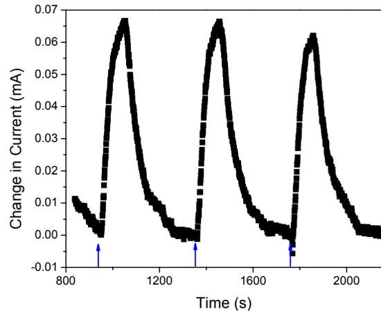
Fig 4. Source-drain current response of an AlGaIn/GaN HEMT sensor exposed to 0.1% diethyl cyanophosphonate in nitrogen. Exposure times are 90 seconds and initiation times are indicated with blue arrows. Measurements were performed at 22°C with a  $V_{ds}$  of 1.5 V.
