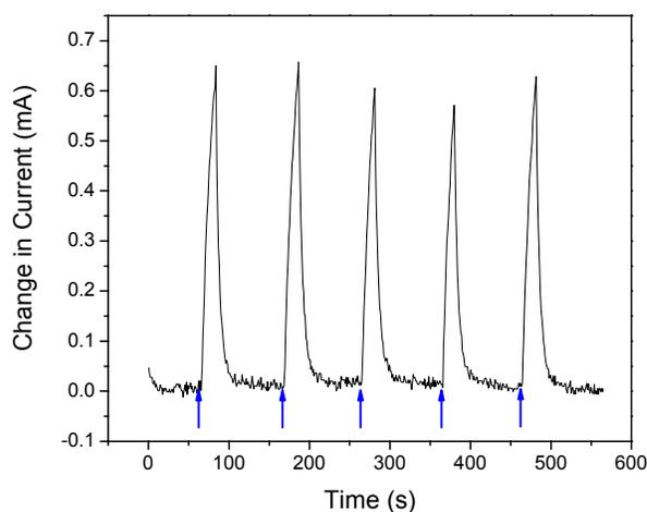
Fig 2. Response of source-drain currents for an AlGaIn/GaN HEMT sensor exposed to mixtures of 1% acetone in nitrogen. The background consists of pure nitrogen and the acetone mixture was added in 10 s exposures (blue arrow). Operating temperature is  $22^\circ\text{C}$  and  $V_{sd}$  is 1 V.
