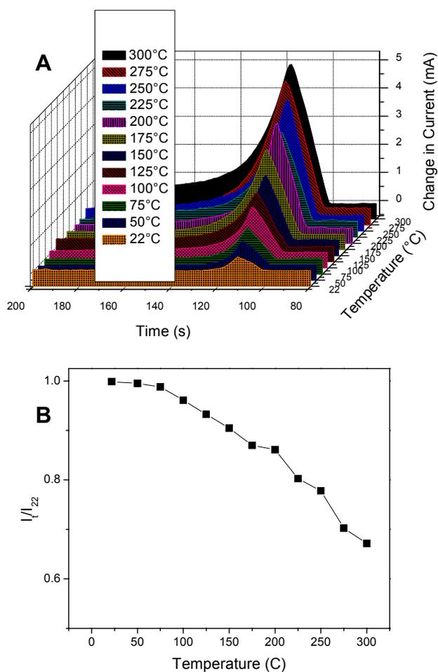
Fig 5. (A) Source-drain current response of AlGaIn/GaN HEMT sensor exposed to 4%  $O_2$  in nitrogen at temperatures from 22°C to 300°C.  $V_{sd}$  is 1 V. (B) Relative source-drain currents for AlGaIn/GaN HEMT under a nitrogen atmosphere. Currents are normalized to the  $I_{sd}$  obtained at room temperature (22°C).  $V_{sd}$  is 1 V.
