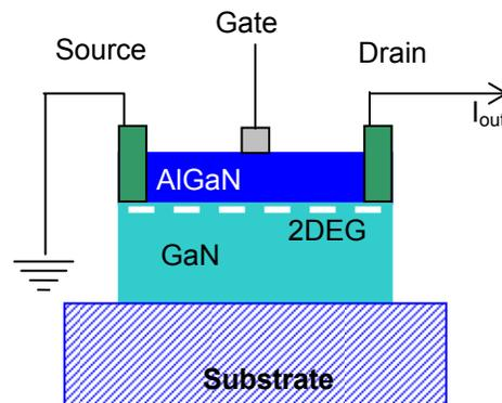
Fig 1. Cross-section of a gas sensitive AlGaIn/GaN HEMT. In the fabricated devices, 4H-SiC substrate is employed with a nickel gate electrode. The AlGaIn and GaN layers are 25 nm and 1  $\mu\text{m}$ , respectively. Channel length is 2  $\mu\text{m}$  and the gate width is 0.15  $\mu\text{m}$ .
