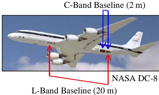
Figure 1: Photograph of the NASA DC-8 showing the positions of the AIRSAR antennas used for ATI.
