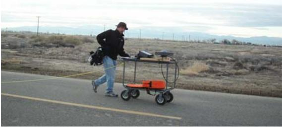
Figure 9: Photograph of a pedestrian control target during the 6 December 2004 data collection. The GPS equipment is on the electronics cart.
