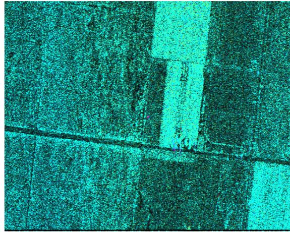
Figure 3: Sample four look C-Band full-baseline along track interferogram showing a control target. Increasing range is to the left of the image. The aircraft's flight direction is down the page. The area represented covers 1630 m in range and 1060 m in azimuth.
