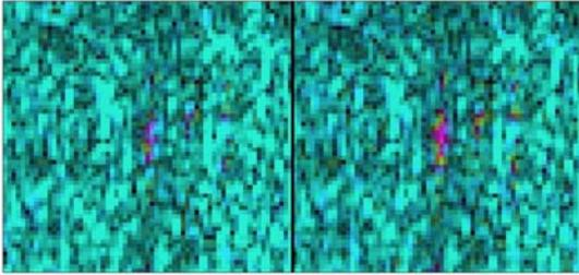
Figure 10: L-Band interferograms imaging the pedestrian pushing the electronics cart. The image on the left corresponds to the interferometric pair with the shorter baseline while the image on the right corresponds to the longer baseline. Each interferogram displays 216.5 m in range and 40.625 m in azimuth. For each chip, range increases across the page while platform flight direction is down the page.
