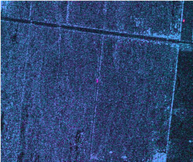
Figure 5: Full-baseline L-Band interferogram centered at position of a target moving predominantly in azimuth. The area imaged covers 1524 m in range and 1025 m in azimuth. The pickup truck shown in Figures 2, 3, and 4 appears as the orange dot in the upper right corner of the image.
