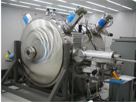
Figure 2. 2 m diam., 2 m long Ultra-high vacuum chamber at JPL showing Nano-Newton Thrust Stand inside chamber.
