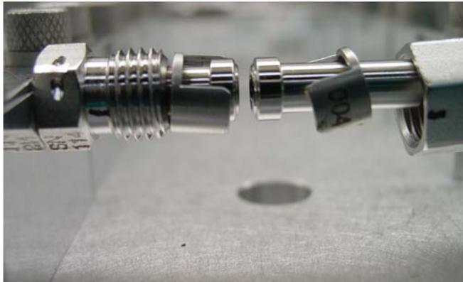
**Figure 2. 1/8 inch Fitting Assembly: Setup showing gland separation distance.**
