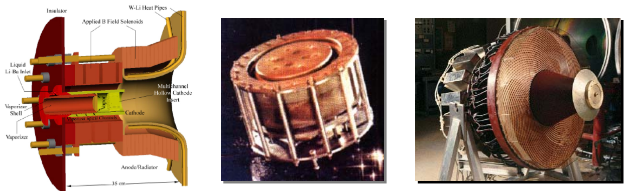
Figure 8. Left: Cutaway view of the Advanced Lithium-Fed, Applied-field Lorentz Force Accelerator (ALFA 2 ) design. Middle: The Very High Specific Impulse Thruster with Anode Layer (VHITAL). Right: The Pulsed Inductive Thruster (PIT).
