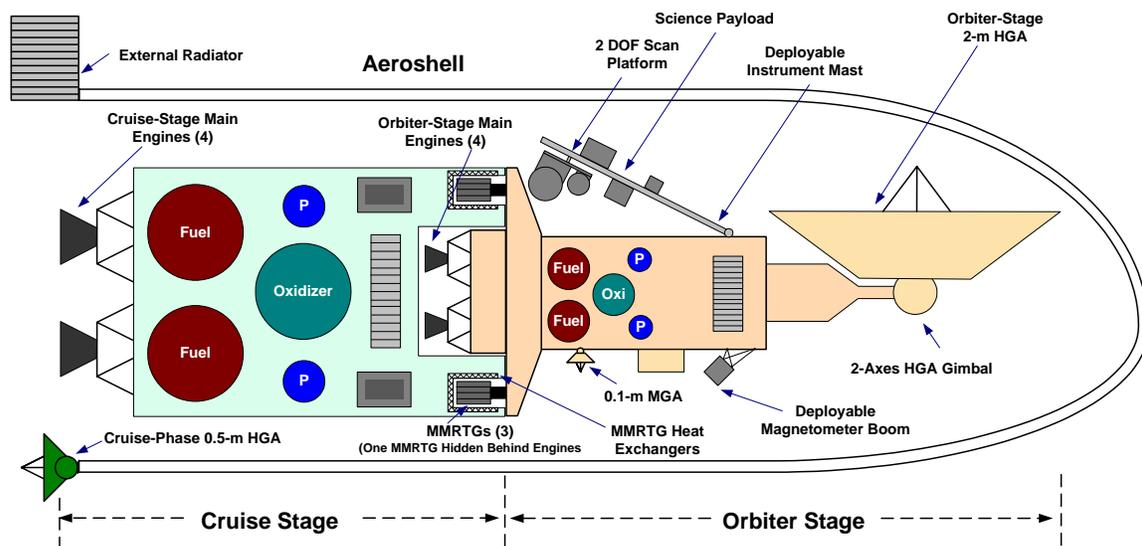
FIGURE 2. Conceptual Illustration of the SRO Spacecraft and Aeroshell
