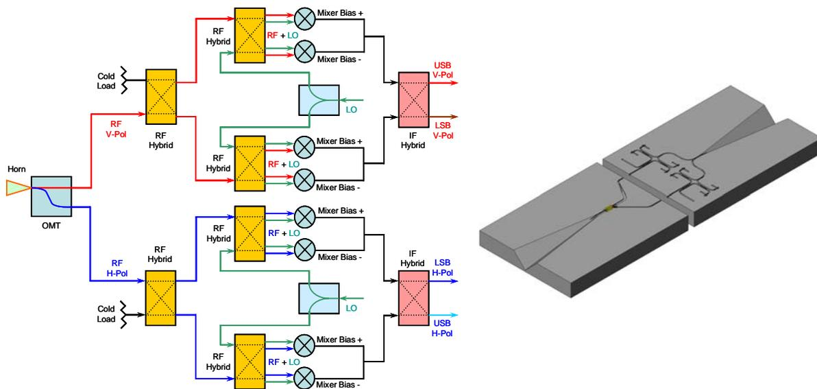
Fig. 1. Schematic diagram of the ultimate heterodyne receiver at submillimeter wavelengths with compact architecture which will enable array integration. This dual-polarized, sideband-separating, balanced receiver can be fabricated using silicon micromachining techniques. The figure on right shows a potential silicon micromachined split-block.
