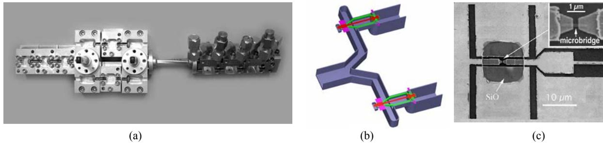
Fig. 2. Pictures of the LO and mixers: (a) 1500 GHz four-stage frequency multiplier chain; on the left are the MMIC power amplifier modules and on the right are the four cascaded doublers [17], (b) proposed frequency multiplier and power combiner module, and (c) HEB mixer with twin-slot antennas [21].
