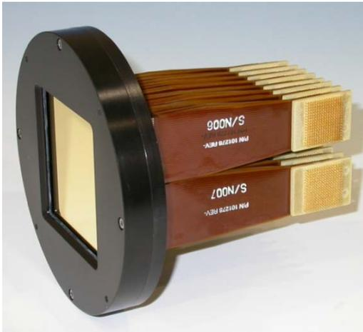
**Figure 8. Deformable Mirrors, Xinetics, Inc. 64x64 actuator model**
