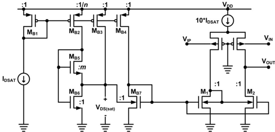
Figure 6. Schematic of a body-driven OTA utilizing a body-driven differential pair and body-driven current mirror
