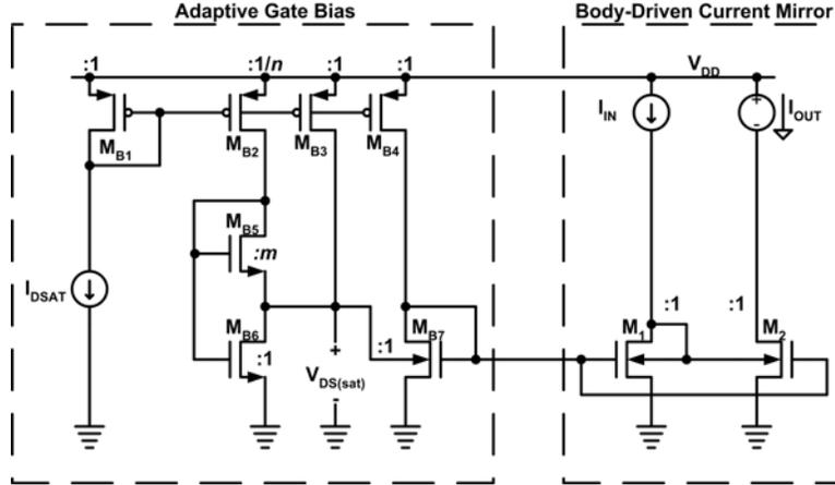
Figure 5. Adaptively biased body-driven current mirror
