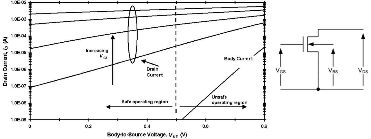
Figure 2.  $I_D$ - $V_{BS}$  at several  $V_{GS}$  values for an (8/0.5) M=16 body-driven nMOSFET and schematic ( $V_{DS} = 1$  V)
