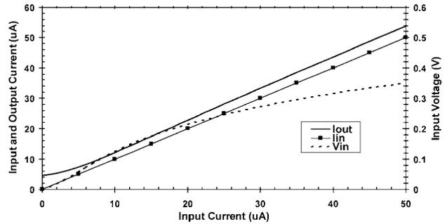
**Figure 8.** Measured  $I_{OUT}$ - $I_{IN}$  transfer characteristic for the adaptively biased body-driven current mirror.  $I_{DSAT}$  is equal to 5  $\mu$ A.
