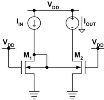
Figure 3. Schematic of a body-driven current mirror with static gate bias [9]
