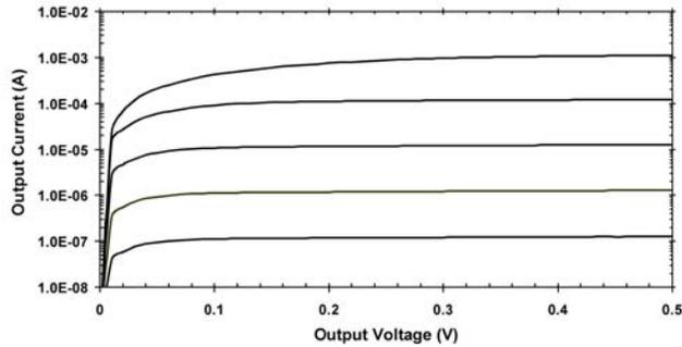
**Figure 7.** Measured  $I_{OUT}$ - $V_{OUT}$  for the body-driven current mirror. In this measurement  $I_{DSAT}$  equals  $I_{IN}$  and is stepped by decades from 100 nA to 1 mA.
