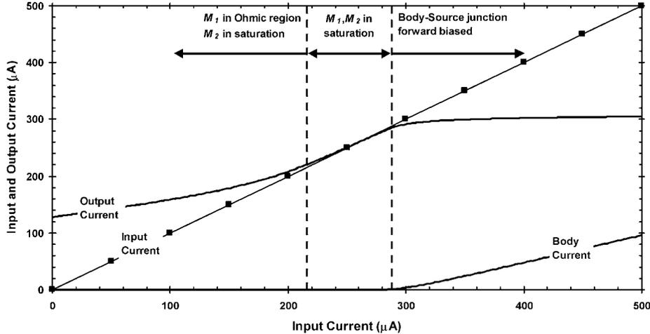
Figure 4. Simulated  $I_{OUT}-I_{IN}$  transfer characteristic for the body-driven current mirror shown in Figure 3.
