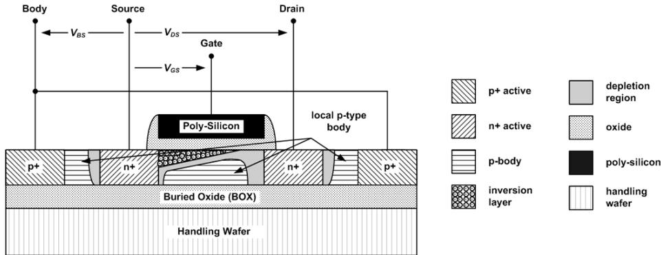
Figure 1. Cross-section of a PD-SOI MOSFET biased in strong-inversion saturation
