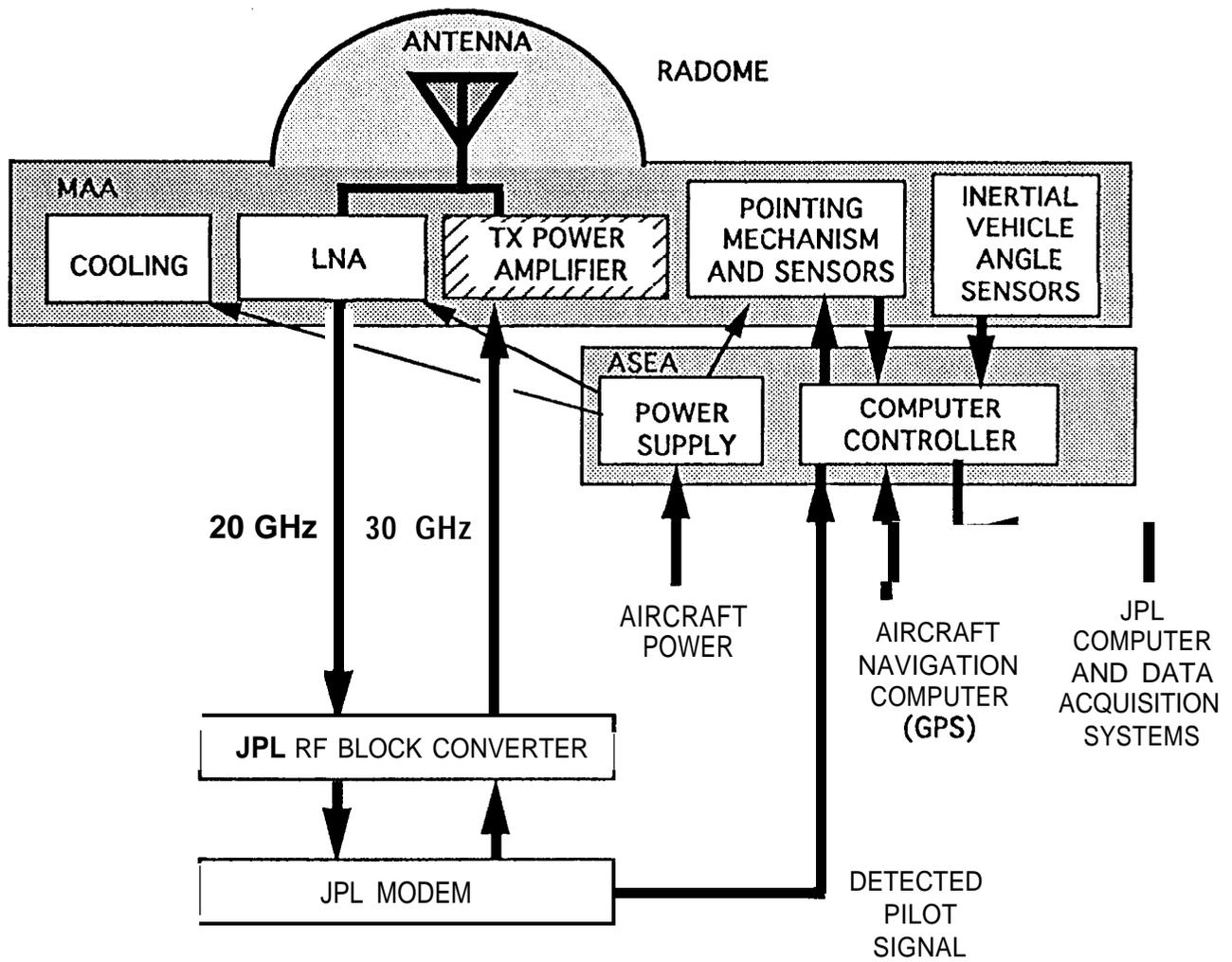
Figure 1. Block Diagram of Broadband Aeronautical Terminal Antenna System
