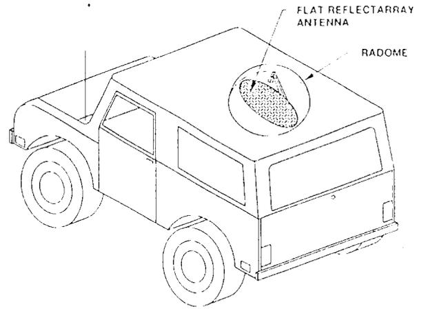
Figure 5. Satellite tracking mobile reflectarray.
