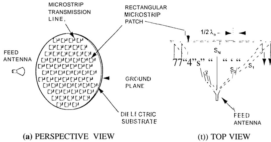
Figure 1. Microstrip reflectarray configuration
