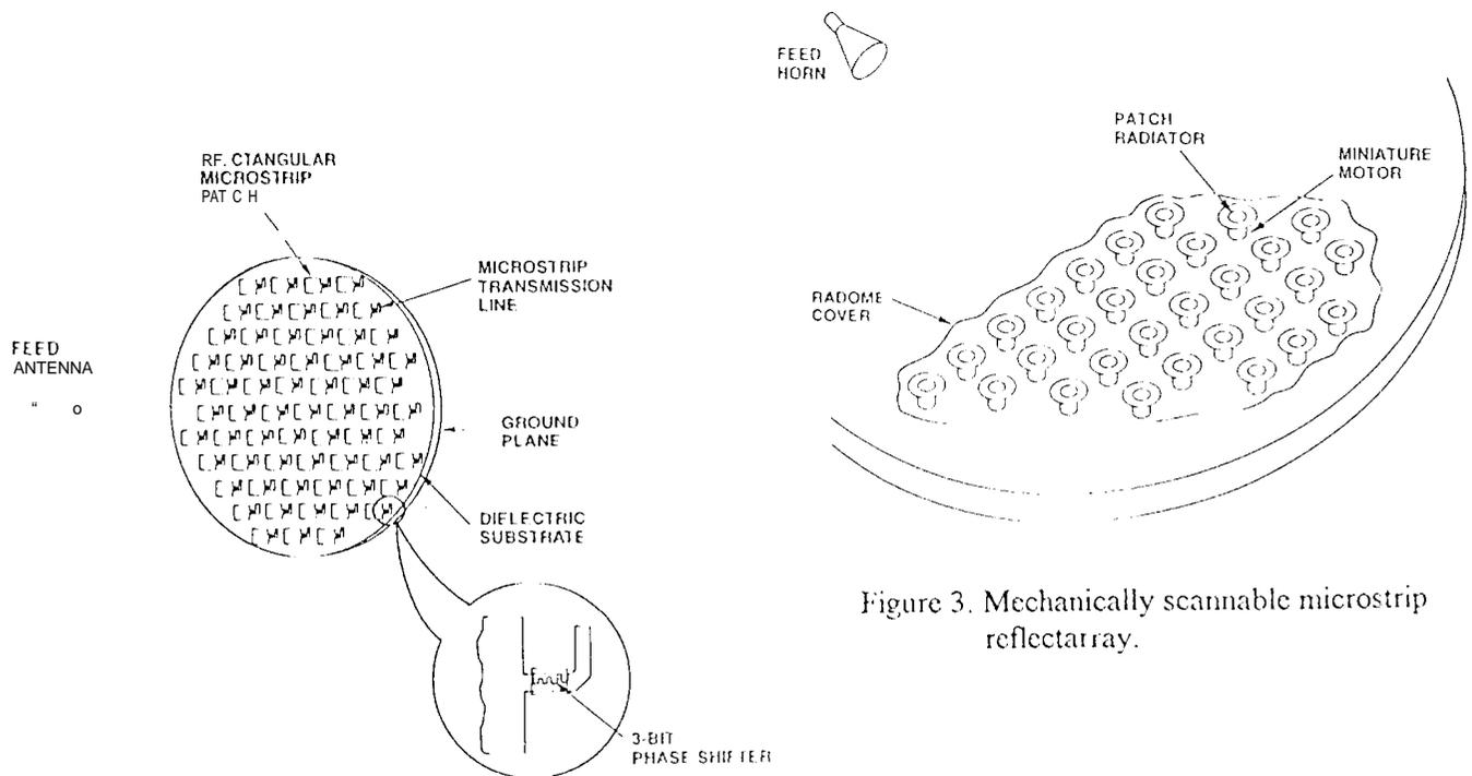
Figure 2. Electronically scannable microstrip reflectarray.
