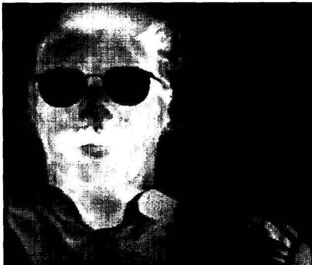
Figure 7(a). A man's face with a warm mustache which was heated by a hot air blower. It also shows the hot air emanating from the air blower. Figure 7(b) shows a cold hand of a person who momentarily held a cold soda can. These images demonstrate the high sensitivity of the 640 x 484 long-wavelength QWIP staring array camera.
