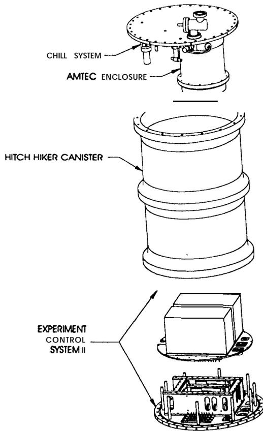
FIGURE 3: APE HARDWARE EXPLODED VIEW
