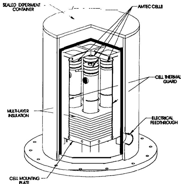
FIGURE 1: AMTEC FLIGHT EXPERIMENT CONCEPT
