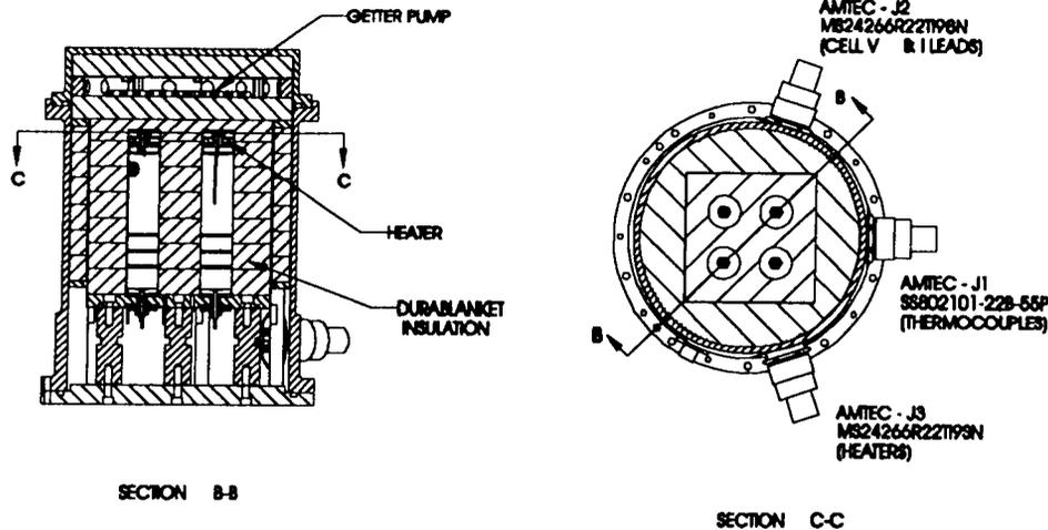
FIGURE 5: AMTEC ENCLOSURE DIAGRAM
