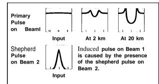
Fig, 2. Computer simulation results for the case of a 20 ps pulse (the shepherd pulse) co-propagating with a 200 ps pulse (approximating a cw primary pulse) in a 20 km dispersion shifted fiber with negligible walkoff. A dip on the 200 ps pulse appeared at the end of the fiber indicating the presence of the shepherding effect.
