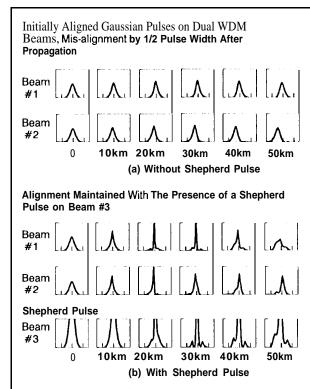
Fig. 1. Evolution of two initially aligned gaussian pulses on the WDM beams. (a) After propagation, separation occurs for pulses on beam #1 and beam #2 without shepherd pulse on the third beam.(b) Alignment maintained for pulses on beam #1 and beam #2 with shepherd pulse on the third beam.
