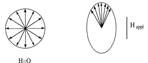
If we first compress the material, the compression rotates some of the moments perpendicular to" the applied stress. When an external field is applied, more moments are then rotated parallel to the field, resulting in larger saturation strains than in an unstressed material [2].
