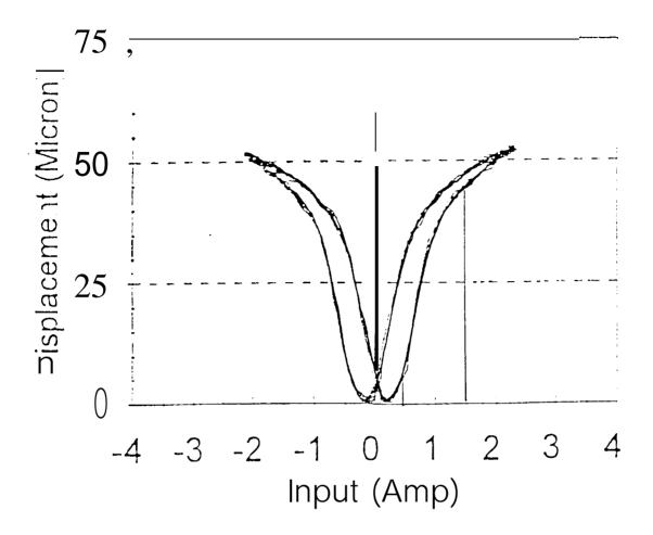
This plot shows the length change of the Terfenol-D crystal in the actuator as a function of applied current at room temperature. (supplied by Etrema)
