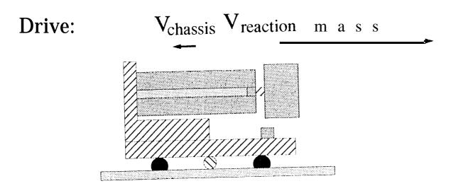
The current (producing a magnetic field) is applied abruptly, driving the reaction mass rapidly opposite the desired direction of motion. The force required for the rapid acceleration is sufficient to cause the bearings to slip along the rails. Conservation of momentum causes the cart to move slightly in the desired direction.
