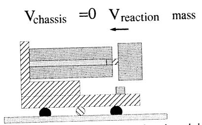
The reaction mass is brought slowly back to its original position. The friction of the bearings on the rails holds the entire assembly in place.
