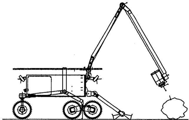
Figure 3: Selected arms for Rocky 7. The shorter arm can dig, grasp *instruments/samples*, and point a spectrometer. The *longer* arm serves as a *multispectral* stereo imaging mast, as *well as* a science instrument placement mechanism.
