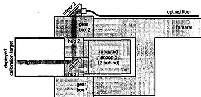
Figure 7: The **lightpath** for the spectrometer through the dual scoop end-effector. The aperture in hub 1 is only open when the scoops are back to back. The calibration target is **usually** stowed in the inner perimeter of the forearm. When the scoops are rotated together through 360 degrees, a tab on the target support (near the hub) is caught by one of the scoops, forcing it to **deploy**. A reverse motion stows the target.
