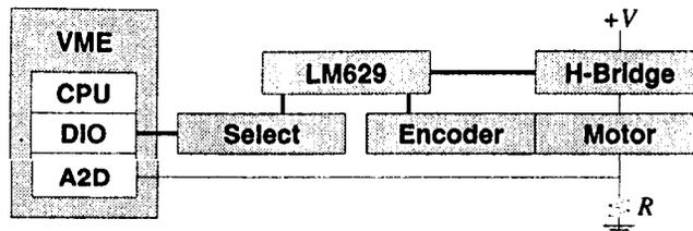
Figure 10: Block diagram of servo level motor control.
