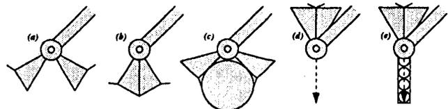
Figure 6: Scoop positions for a variety of operations: (a) digging and dumping, (b) **sample** enclosure, (c) instrument grasping, (d) spectrometer pointing through opened **aperture**, (e) spectrometer calibration target deployment.
