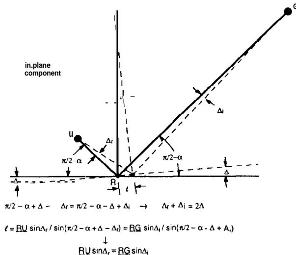
**Fig. 4. Adjustment of reflection point on sea surface due to the deviation of normal vector from geocentric radial vector: ORG plane component**
