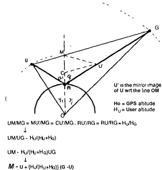
Fig. 3. Geometry of GPS (G), User (U) and reflection point (R)
