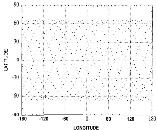
Fig. 2. Geographic coverage of conventional Topex altimetry measurements over 1 day at 2-minute intervals
