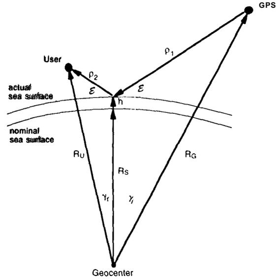
Fig. 6. Determination of altimetry height h from reflected GPS to User range measurements
