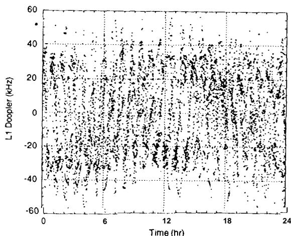
Fig. 10. Doppler shift of reflected GPS signals observed by Topex over 1 day at 2-minute intervals
