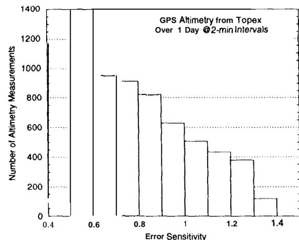
Fig. 9. Sensitivity of sea surface height determination to reflected GPS range measurement error
