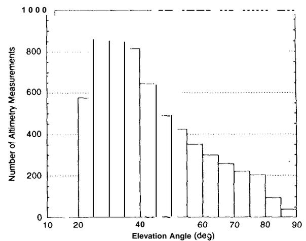
Fig. 8. Elevation angles at the sea surface reflection points
