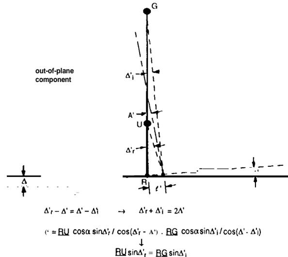
**Fig. 5. Adjustment of reflection point on sea surface due to the deviation of normal vector from geocentric radial vector: component in a plane orthogonal to ORG plane**
