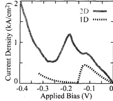
Figure 3: simulated hole RTD I-V characteristics. 2D simulation according to Eq. (1). 1D simulation according to Eq. (3) significantly underestimates the current.
