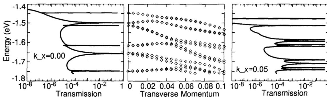
Figure 2: RTD hole subband dispersions at zero bias and two selected transmission coefficients at  $k=0$  and  $k=0.05$ . The subband dispersion shows strong band mixing and anti-crossing. The transmission coefficients show a correspondingly strong dependence on transverse momentum  $k$ .
