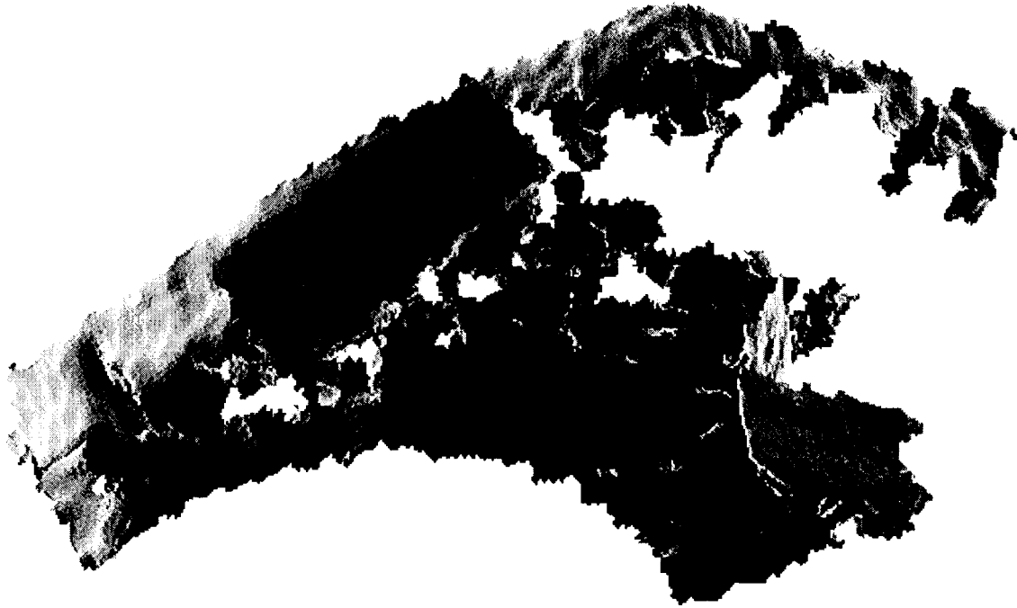
Figure 5: Sample Integrated Surface Map Thirty two individual range maps have been registered and integrated into a single coherent surface. Obvious features include the far wall in light grey, an occluding planar piece of sheet metal resting against the wall in the middle of this image, and the corner of a large concrete cube in light grey on the near right.
